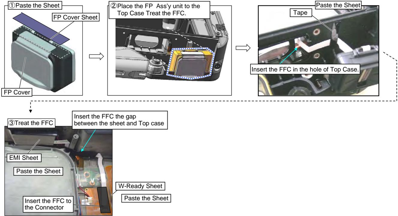
**Install the Handle Base (FP) and SP Ass'y parts**
